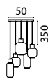
2162-85-05GL-50-5 Black Fixt. Brushed Brass Cover, Fabric cable, 5x E27 max 18W Bulb excl.
